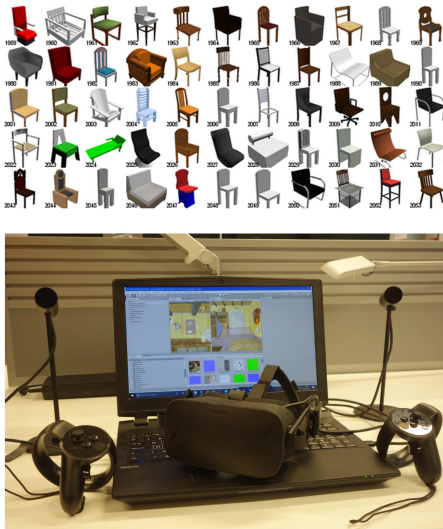
Figure 1: Our approach searches a dataset of chair 3D models (top left) using free-hand drawn sketches within a virtual reality. Our setup consists of Oculus RIFT, Oculus Touch and a laptop (bottom left). Sketches can be made either on top of a template chair or a prior search result (right).
