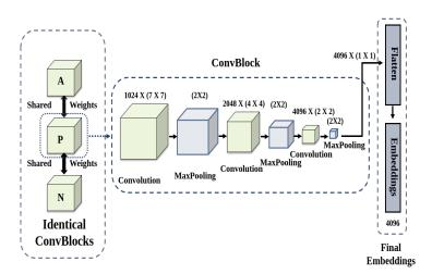
Fig. 4. Our ConvBlock takes in the encoding from fig. 2. The ConvBlock consists of a network of convolutional and maxpooling layers, which pool the spatial information and merge the foreground and background encodings to obtain final embeddings.
