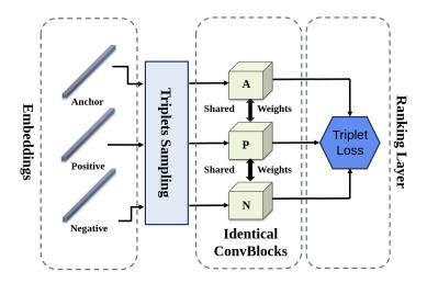
**Fig. 3.** Triplet of input tensors corresponding to images. Each tensor contains an embeddings of the anchor image A, positive image P and a negative Image N which are fed into three identical deep neural networks independently with shared weights where the triplet loss is optimized.
